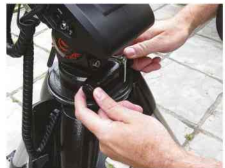
▲ Drift alignment involves making small adjustments to the azimuth and altitude bolts
